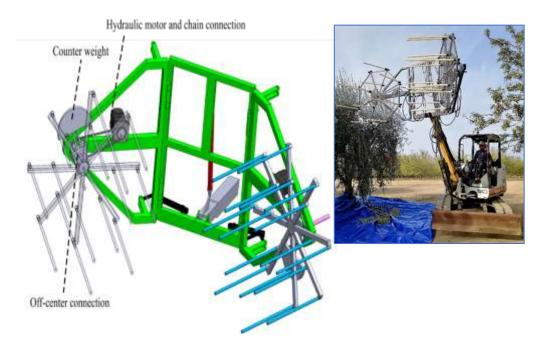
**Figure 7.** UC Merced canopy contact harvester head.
