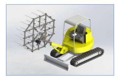
Figure 14. Proposed shaker design with a side-mounted canopy shaker.
