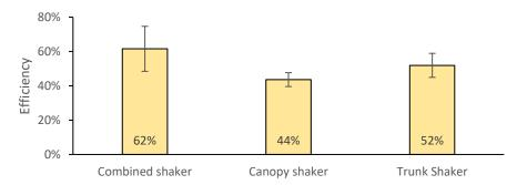
**Figure 13.** Average harvest efficiency for three methods demonstrating the average higher efficiency when the trunk and canopy shaking are combined.
