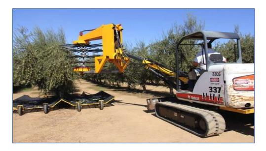
**Figure 2**. A canopy contact harvester adapted from a jatropha harvester. Canopy contact harvesters have higher potential efficiencies with hedgerow orchards that can present a hedgerowed vertical fruiting wall to the harvester head. These orchards can be developed from existing orchards at, 96 -139 tree per acre, with mechanical pruning or developed as a hedgerow at higher densities, 202 trees per acre.
