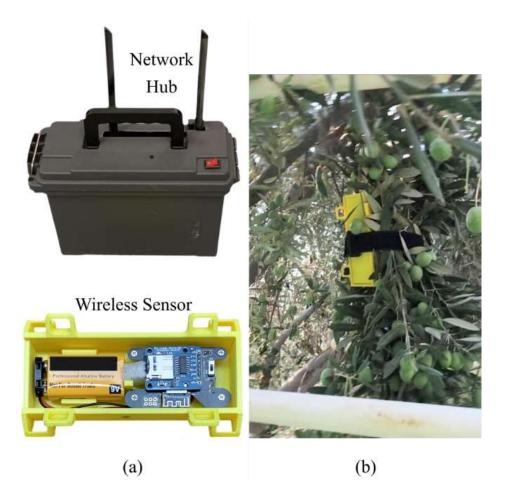
**Figure 8**. Wireless sensor module and network hub (a) and wireless sensor module installed on olive branches for data collection (b).
