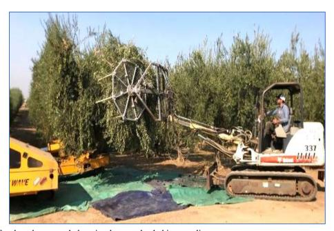
Figure 11. Trunk and canopy shaker simultaneously shaking an olive tree.
