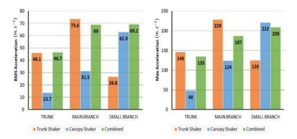
**Figure 9**. Root mean square or vibration at each part of the tree (left) and maximum acceleration produced by the two harvesters alone and together within each part of the tree (right).
