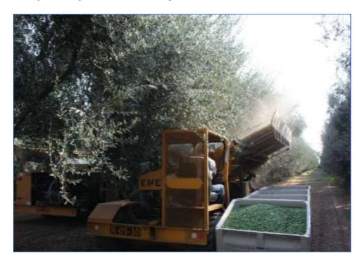
**Figure 3**. Double sided trunk shaking pistachio harvester that can be used in existing orchards, 96 -139 tree per acre, modified with mechanical pruning or hedgerow orchards at higher densities, 180-202 trees per acre.
