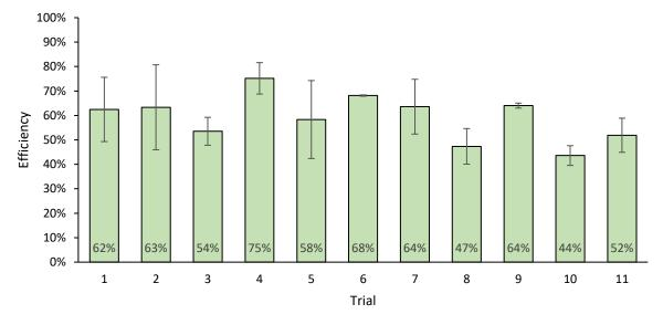
**Figure 12.** Harvest efficiency for all 11 trial combinations. Trials 1-9 used the canopy contact and trunk shaker simultaneously. Trial 10 used the UC Merced Canopy shaker alone and trial 11 used the OMC trunk shaker alone.
